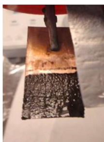
Fig. 1: The obtained deposit after 5h at 5.25V, 0.01A
